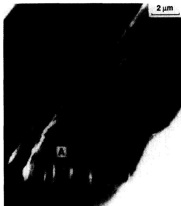
Figure 4 Morphology of kink bands 1.2\text{--}1.8\ \mu\text{m} thick showing uniform band thickness and voids in the bands. (The longitudinal cracks are probably due to splitting during specimen preparation)
