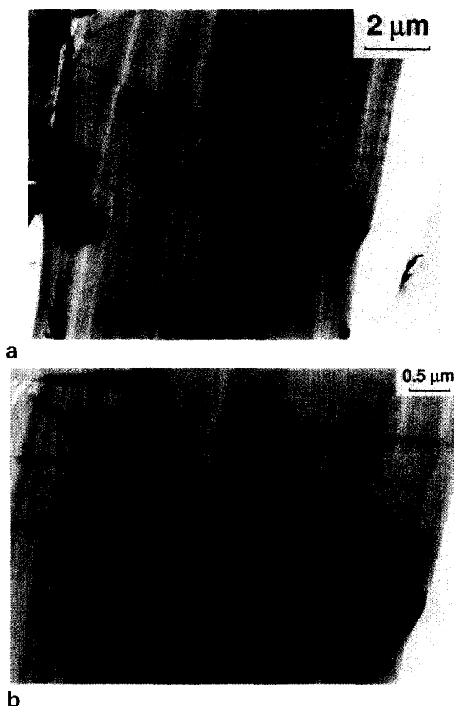
Figure 5 (a) A band with intermediate thickness ( 0.1\text{--}0.3\ \mu\text{m} ) showing a step on the surface and variations in band thickness along its path. (b) An enlarged view of the step and the band showing the irregularity of the band thickness and boundaries along the length
