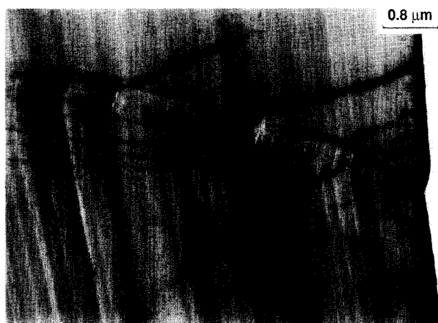
Figure 3 A step on the fibre surface with a kink band extending from it. The band is wavy in its path and non-uniform in thickness
